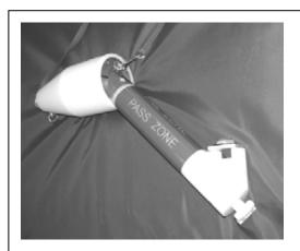
Figure 5. Cone and cylinder tool.
