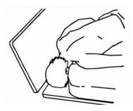
Zone 7 is the space between the inside surface of the head board or foot board and the end of the mattress. This space may present a risk of head entrapment when taking into account the mattress compressibility, any shift of the mattress, and degree of play from loosened head or foot boards. FDA recognizes this area as a potential for entrapment and encourages facilities and manufacturers to report entrapment events at this zone.
