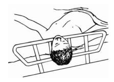
Zone 1 is any open space within the perimeter of the rail. Openings in the rail should be small enough to prevent the head from entering. A loosened bar or rail can change the size of the space. The HBSW and IEC recommend that the space be less than 120 mm (4 <sup>3</sup>/<sub>4</sub> inches), representing head breadth.
